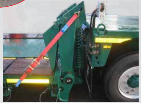
Double ramp for front loading
