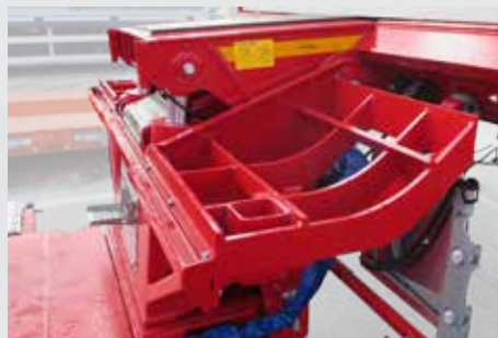
Wheel recess on the gooseneck
