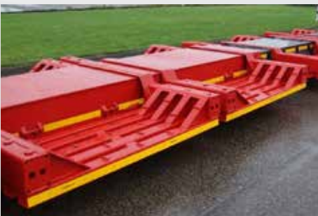
Turnable wheel-recess for center spine
