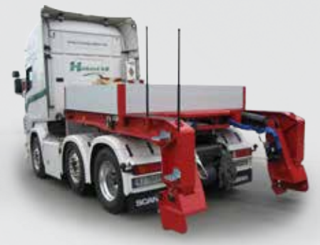
Detachable gooseneck with outer beams
